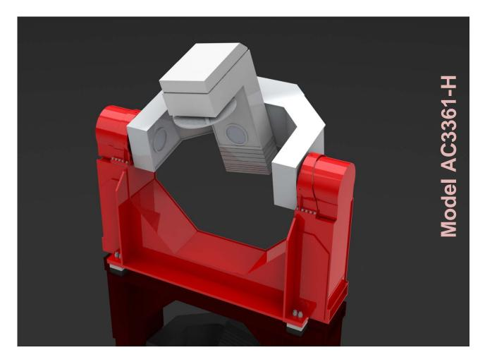
The AC3361-H is designed to accommodate gyro-stabilized optical pods such as FLIRs, target designators or camera systems. The large inner axis (yaw) platform supports the payload or Unit Under Test (UUT). To keep the test article's focal point at the axis intersection a large offset is necessary. The Harmonic drives are chosen for their low backlash, high gear ratio and compact size.
