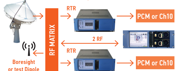
RSR-RF implementation in a station
