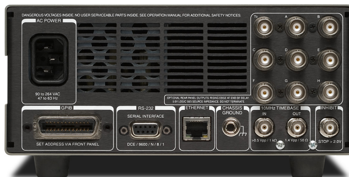
DG645 rear panel with Opt. 01 outputs
