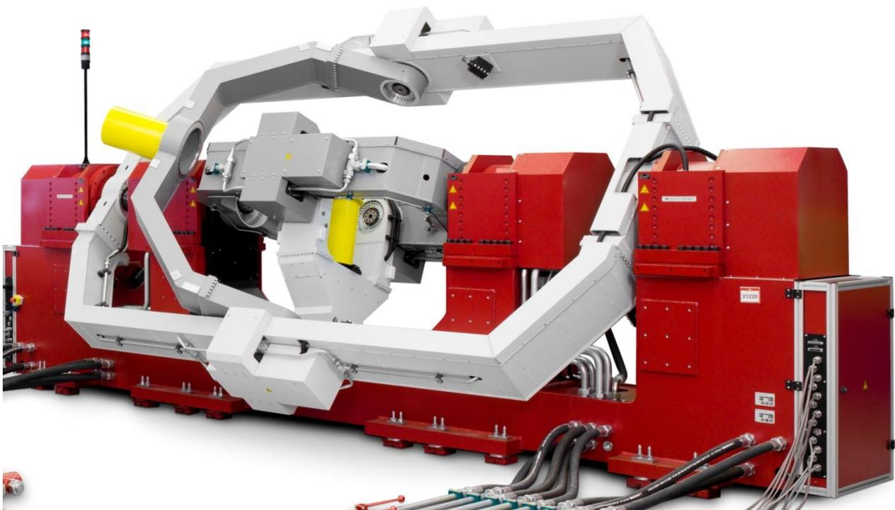
The HD55H-T35.50 is a precision 3-Axis Flight Motion Simulator (FMS) combined with a 2-Axis Target Motion Simulator (TMS). The system is specifically designed for the Hardware-in-the-Loop (HWIL) testing and evaluation of high dynamic Infra-Red and Electro-Optical missile systems and sensors.
